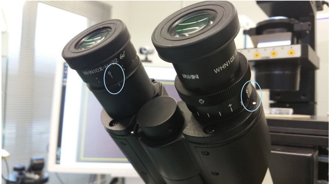
Fig. 56: Diopter adjustment (example: Olympus inverted microscopes)
